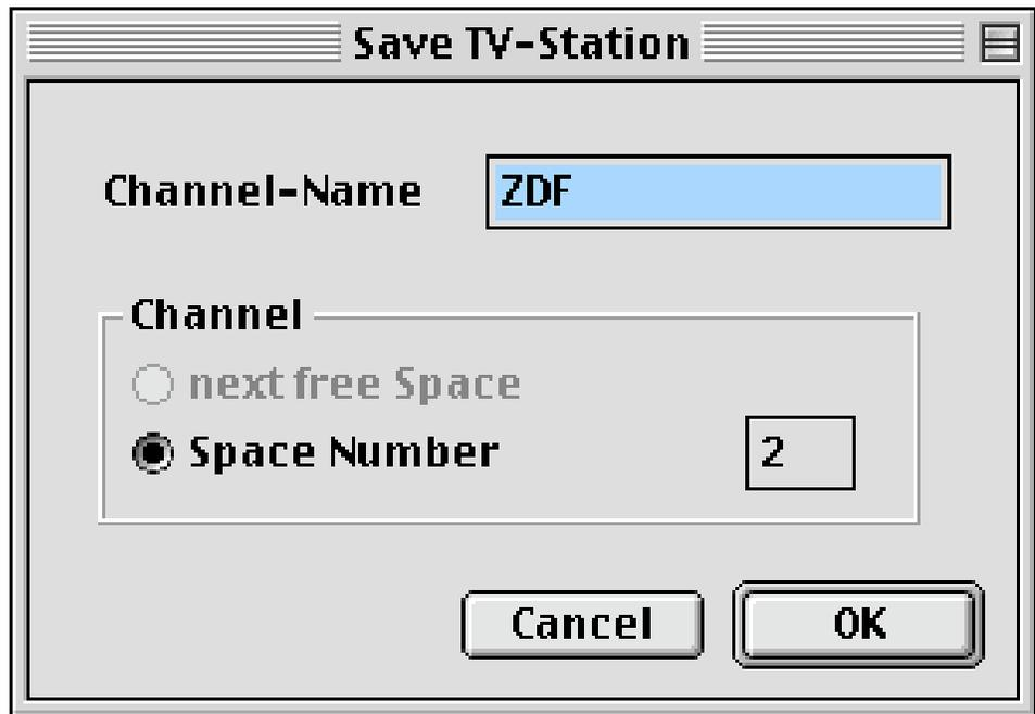
In this dialog box it is possible to enter a name for the station which is to be saved and to choose if it should be saved in the next available slot or one to be chosen freely. The field in which the number can be entered can always contain the next available number when it is called up. Unless, of course, only the fine tuning of an active channel has been changed. In this case the actual number and name are entered. The possibility to use the next available number is blocked.
